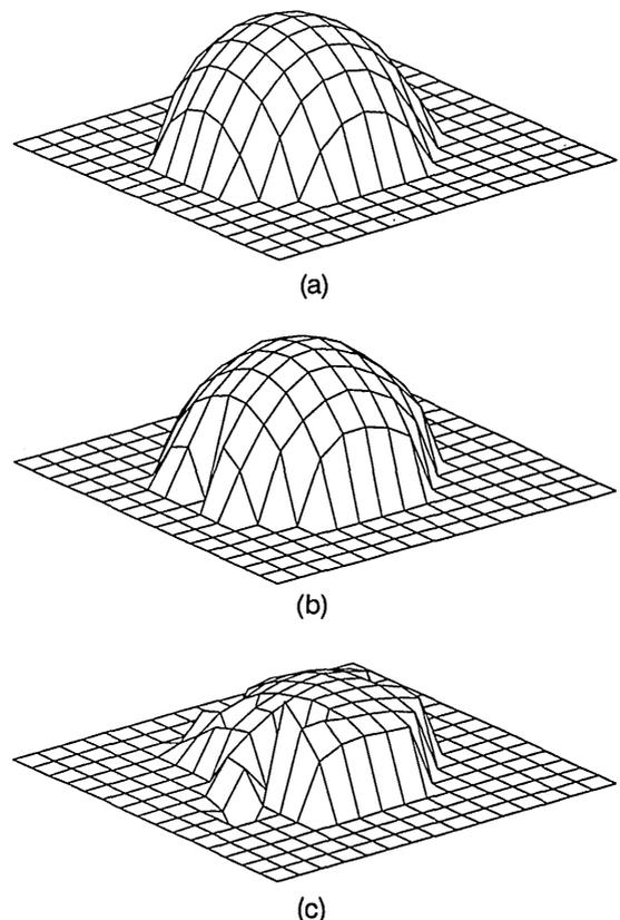
Fig. 3. Reconstructed shape of a spherical surface from the computer-generated image for different levels of noise: (a)  $\sigma = 0$ , (b)  $\sigma = 0.2$ , (c)  $\sigma = 0.4$ .
