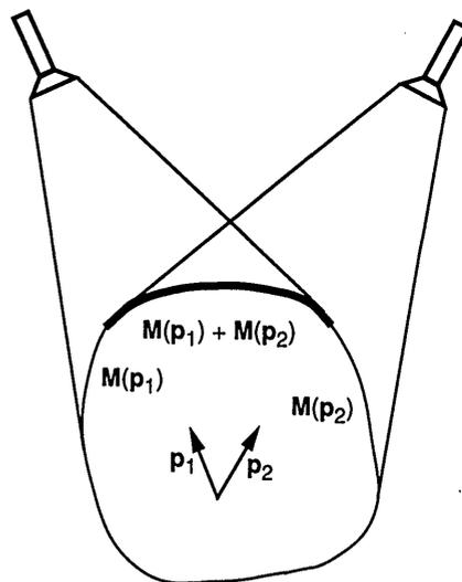
Fig. 1. Arbitrary surface illuminated by two light sources ( $\hat{p}_1$  and  $\hat{p}_2$ ). The region outlined by the heavy black line is illuminated by both sources simultaneously. In this region  $\mathbf{M} = \mathbf{M}(\hat{p}_1) + \mathbf{M}(\hat{p}_2)$ .
