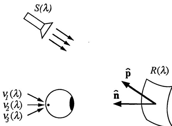
Fig. 1. Small patch of matte surface illuminated by a point light source with spectral power density function  $S(\lambda)$ ; the direction at the light source is  $\hat{p}$  (unit vector). The orientation of the surface is defined by unit normal  $\hat{n}$ , and its reflectance properties by spectral reflection function  $R(\lambda)$ . For every point of the receptive surface, three different receptors with spectral sensitivities  $\nu_i(\lambda)$  are present.
