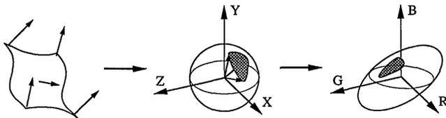
Fig. 2. Mapping of surface normals (left) onto trichromatic response space (right) can be considered the superposition of the mapping of surface normals onto a Gaussian sphere (middle) and the mapping of the Gaussian sphere onto response space (right). The images of the surface normals on the Gaussian sphere and its image (ellipsoid) in the trichromatic response space are depicted by the shaded regions.
