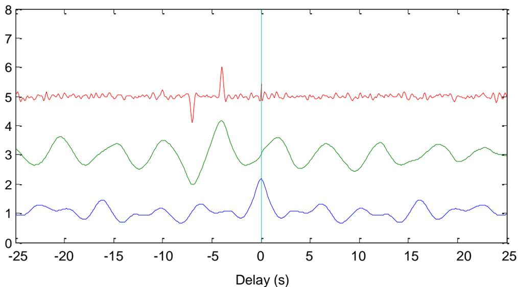
Fig. 12. Autonormalized analysis of inhibitory feedback. ACF of input signal (blue), CCF of output with (iterative) inhibitory feedback (green), and autonormalized CCF (red) revealing the excitatory (4 s) and inhibitory (7 s) delays.
