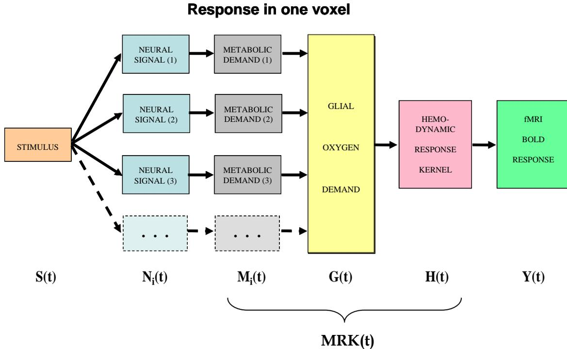
Fig. 1. Block diagram of the main processing stages that lead up to the BOLD signal. The subscript  $i$  indicates that the stage incorporates multiple components within the voxel.
